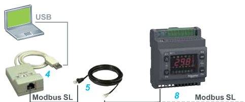
Remote programming - M171 optimized
