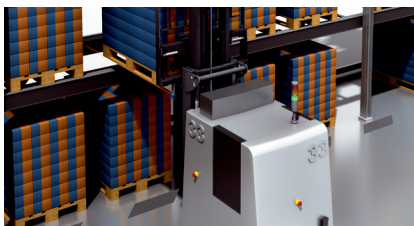
Empty bay detection with automated guided vehicles
