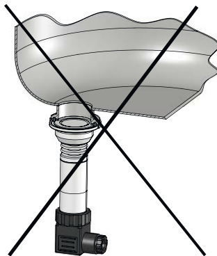
Not self-draining mounting position
