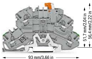
Double-deck disconnect terminal block; with a pivoting knife disconnect; gray housing
