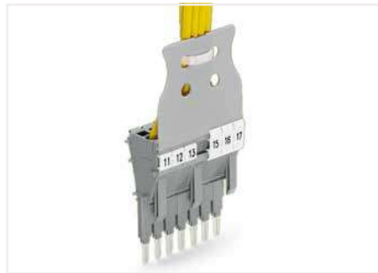
Module assembly with CAGE CLAMP® connections (0.25 ... 2.5 mm 2 /24 ... 14 AWG), including strain relief plate and marker slots for Mini-WSB or WMB markers.
