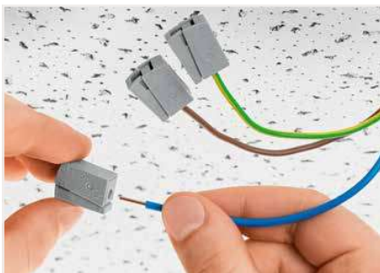
To connect: Insert stripped solid conductor into circular entry and push until it hits the backstop.
