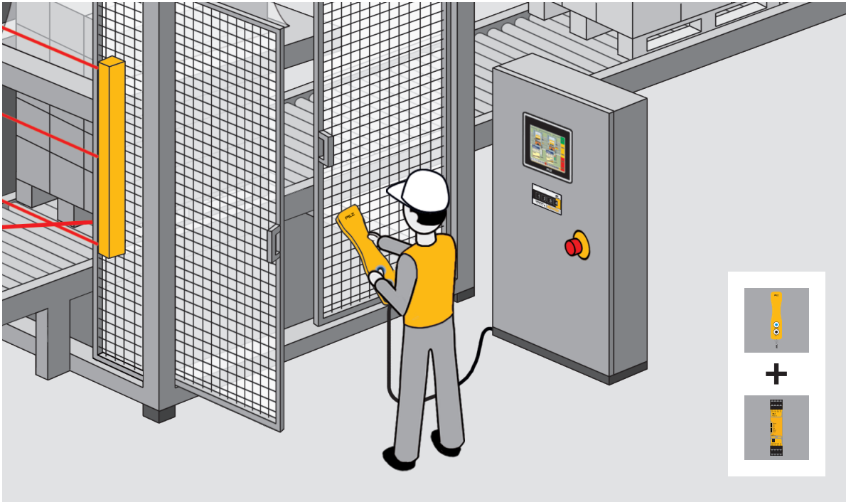
The optimum solution: two-hand monitoring with the manually operated control device PITjog and the safety relay PNOZ s6.
