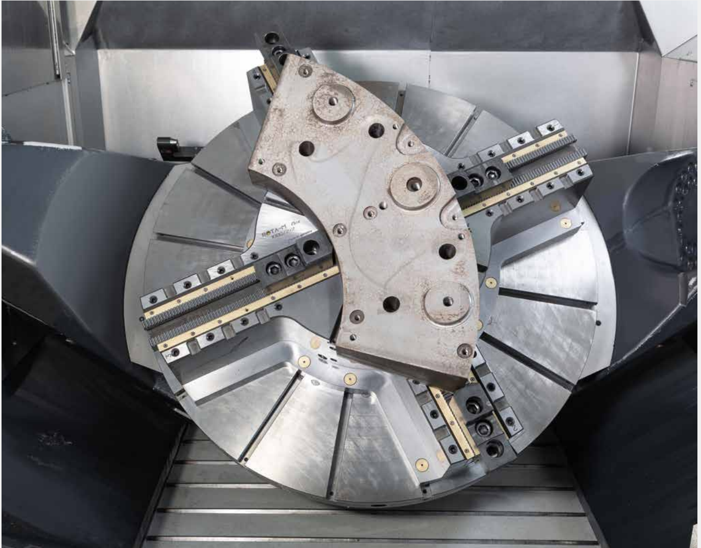
One meter diameter: With the new lathe chuck ROTA-ML flex 2+2 1000 Schumacher can machine all parts specifically and efficiently in its DMU 105 FD mono-BLOCK five-axis machining center from DMG Mori.
