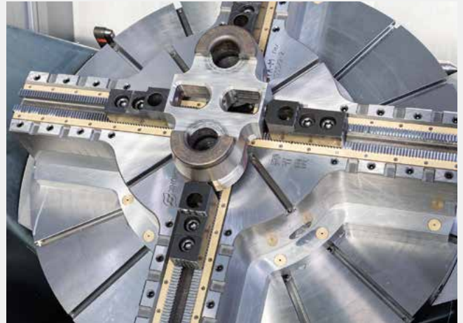
Machining this complex-shaped guide seat for vibrating heads, which shake off sand in the foundry, is no problem for the lathe chuck ROTA-ML flex 2+2.
